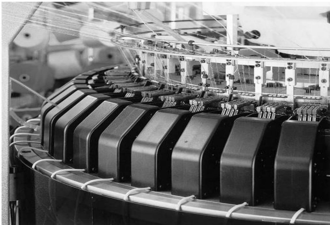
Fig. 1.22 Rib jacquard machine with three –way selection and four –color stripes
